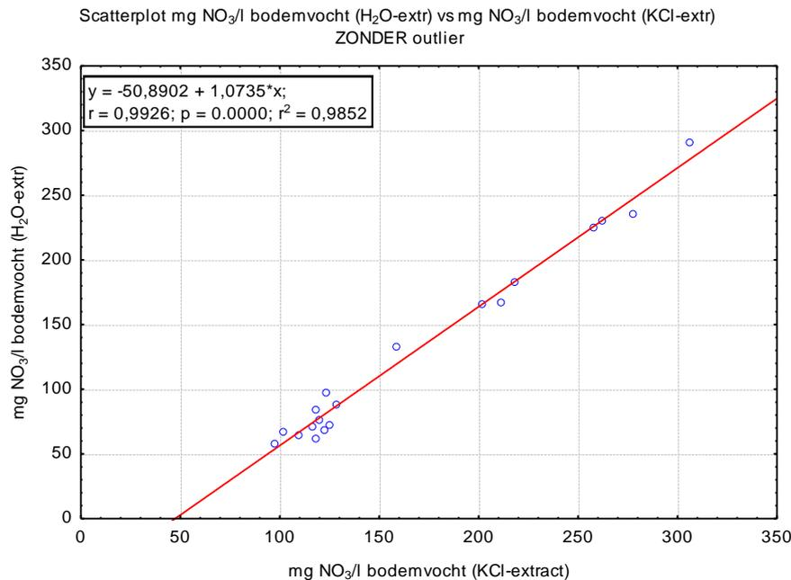
Figure 461: Scatterplot of the nitrate concentration in the soil water determined by extraction in water ( $\text{mg NO}_3/\text{l H}_2\text{O-extr}$ ) versus the nitrate concentration in the soil water determined by extraction in potassium chloride ( $\text{mg NO}_3/\text{l- KCl-extract}$ ). (samples under limit of quantification not withheld)
