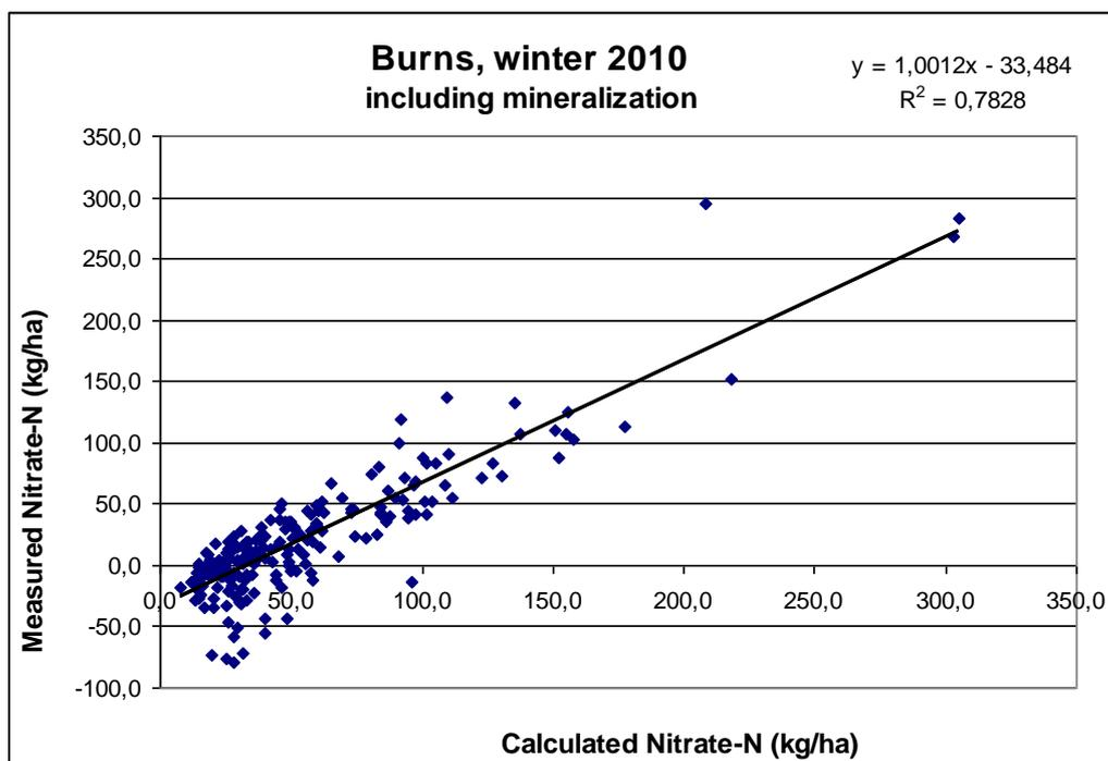
Figure 87: Measured (amount of nitrate before winter in the soil profile – amount of nitrate after winter) amount of nitrate-N (kg N/ha) leached out during winter 2010 versus calculated (Burns model) amount of nitrate-N (kg N/ha) leached out during winter 2010, including corrections for mineralisation.
