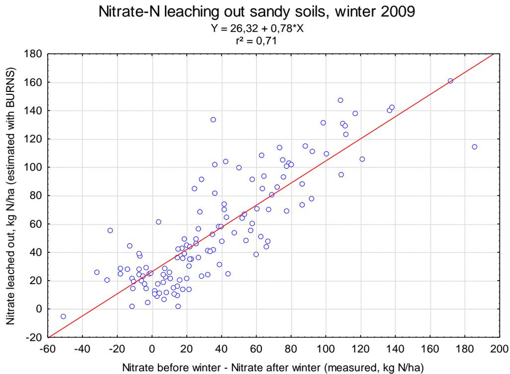
**Figure 83:** Amount of nitrate-N (kg N/ha) leaching out the soil profile estimated with the Burns model versus the difference between the amount of nitrate-N measured before and after winter 2009 for sandy soils.
