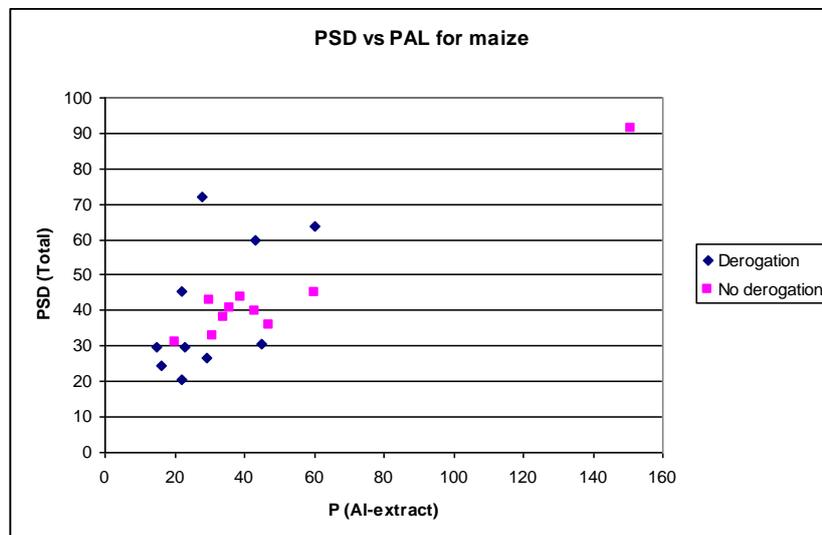
Figure 74: The relation between P (AL-extract) and PSD for derogation ( $R^2=0.30$ ) and no derogation ( $R^2=0.94$ ) parcels cultivated with maize. PAL is measured on soil samples of 2009 and PSD on samples of 2010, both from the same parcels.
