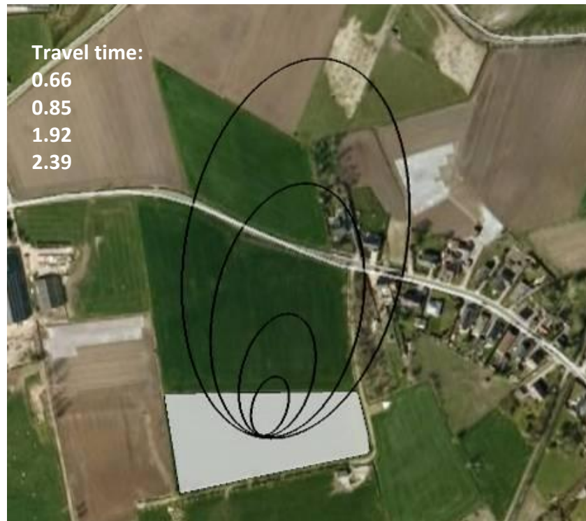
Figure 2: Infiltration areas for hypothetical monitoring wells in the middle of the parcel for different depths. For each depth (0.95m, 1.45m, 2.45m and 3.45m) the travel time is listed.
